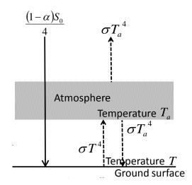
where T is the surface temperature, and  $T_a$  the atmospheric temperature. The heat budget of the ground surface gives
